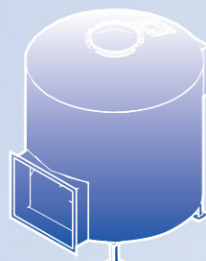
Vertical Structure + Drawer-type Ash Hopper Prevent \text{SiO}_2 blockage measures
